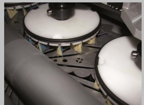
At Bogballe we use Discs for the deburring. Traditional heads can in many cases also be used
