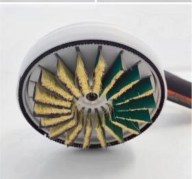
Flex Sander 60 is an industrial brush sanding machine developed by Flex Trim and is a powerful alternative to existing hand sanders.
